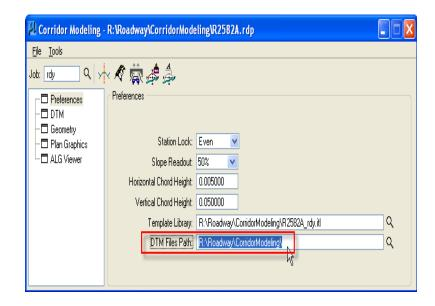
3. The XSC and XPL created from Corridor Modeling should remain in the "CorridorModeling" folder. The proposed DTMs are linked to the ALG and "cmjobRDY.xml" files under the "RDDBS" folder. Other Units such Hydro, Geotech, and Utilities have to be notified of this location for the cross sections Roadway produces.
