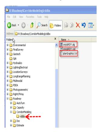
If you have stored the plan graphics in the DSN or EOP DGN file while under the original "Proj" folder, the ALG and planGraphics links are then stored incorrectly in the "RDDBS" folder under it.
